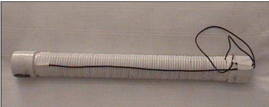
I chose to use the matching method of a series variable capacitor (a mica compression unit rather than a matching transformer or inductive link of one or more turns over the main coil. I think that this is a more efficient way of transferring the power to
