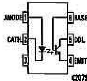
One additional component is needed, a readily available 4n25 optocoupler ([http://www.jaycar.com.au/products\\_uploaded/ZD1928.pdf](http://www.jaycar.com.au/products_uploaded/ZD1928.pdf)), plus a bit of wire. The 4n25 is a 6 pin integrated circuit, and I'm not even going to give a circuit diagram.
