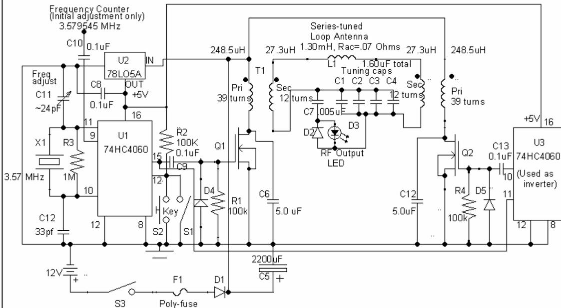
80 WATT PUSH-PULL CLASS-E TRANSMITTER CIRCUIT DIAGRAM
