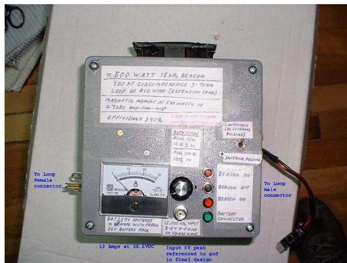
Figure 7—Prototype 500 Watt Beacon Amplifier
