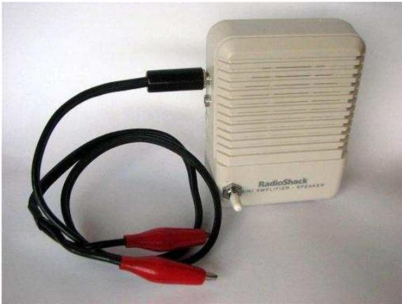
A small amplified speaker attached to the field telephone system can be a useful tool for Incident Command and other locations during a rescue. It allows personnel to receive information without constantly holding a phone to the ear. With this version, headphones can be connected and at the flip of a switch the speaker can be muted for privacy.
