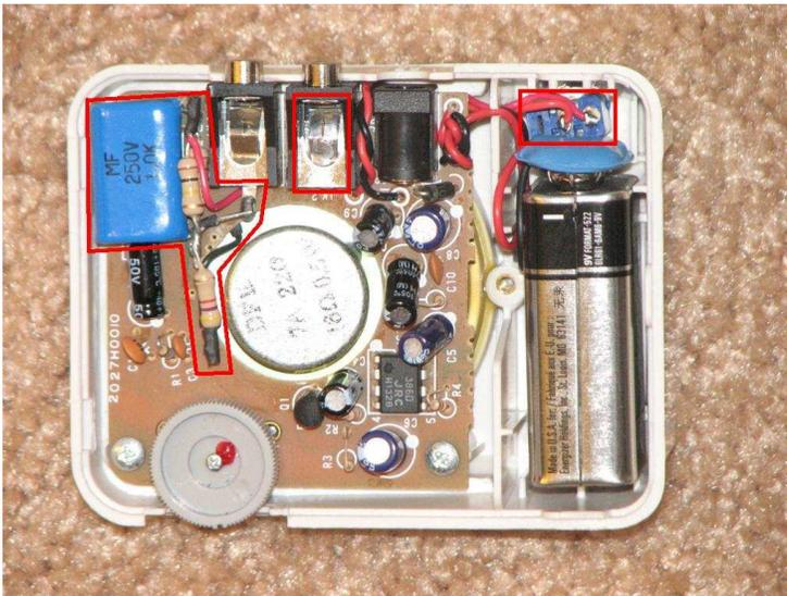
In the right highlighted area I added a mute switch in series with the speaker. Please note this does not turn off the amplifier, it only silences the built-in speaker. Be sure to adjust the volume control to match the type of phones connected to the line. Keep the volume setting low when listening to battery-powered phones, and raise it for sound-powered phones. If a phone is located nearby, consider muting the speaker while transmitting. This will avoid annoying feedback distortion.
