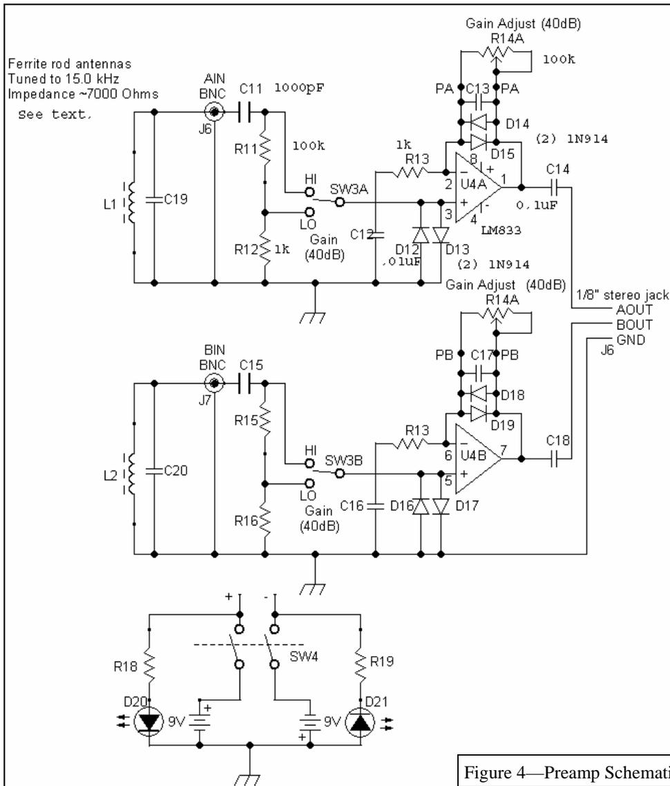
Figure 4—Preamp Schematic
