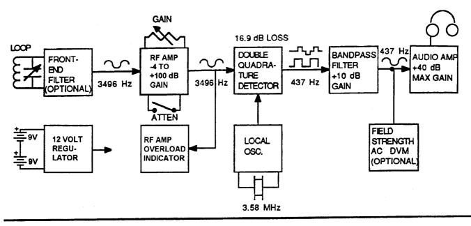
DOUBLE-QUADRATURE DETECTOR AND LOCAL OSCILLATOR USED IN ABOVE RECEIVER ( Dashed lines are the optional PLL circuits)
