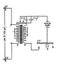
Drawing and circuit of the French "Parleur" power buzzer, model "2 ter". Initially, British power buzzers were made to this design.
