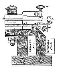
The British "Power Buzzer" was a large electric buzzer with a secondary step-up winding connected to a pair of bayonets stuck into the ground 100 yards (91m) apart. The receiver was a vacuum-tube audio amplifier connected to a similar pair of grounds, 2000-4000 yards away (1.1-2.3 miles; 1.8-3.7 km). To prevent interference, buzzers with different frequencies were manufactured; the operators' ears provided selectivity.
