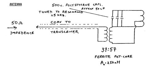
Notes - 1. Square frame, 1.42m across diagonal. Coil is 1 turn of 16/3 outdoor cable connected in series to give 3 electrical turns, tapped at 1 turn.
