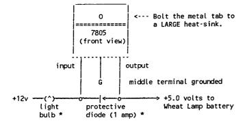
\* = Optional components: A suitably rated lightbulb in series with the regulator would act as a current indicator and dissipate some of the heat that the 7805 would otherwise have to dissipate. A reverse-biased diode across the 7805 will keep it from being damaged in case power is removed with the 4-volt battery still connected.
