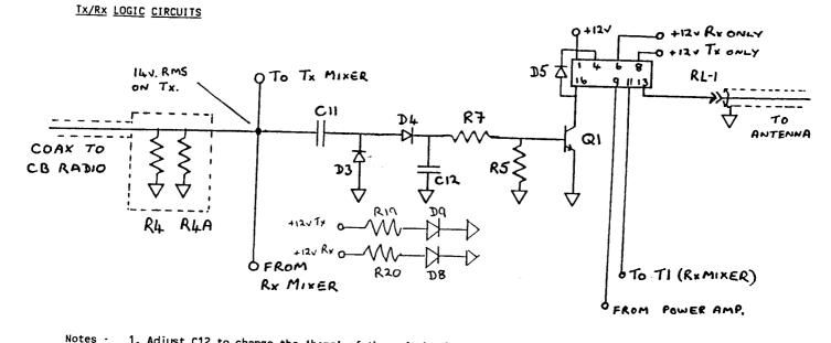
otes - 1. Adjust C12 to change the 'hang' of the switch after releasing the CB radio transmit switch.
