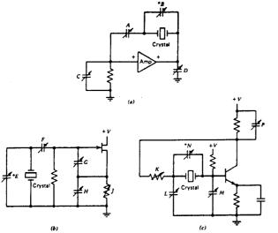
Figure 8.1. Capacitor locations for frequency trimming in three popular oscil-lator circuits. \*Indicates locations that are not recommended. (a) Series resonant, (b) Colpitts, and (c) Pierce.
