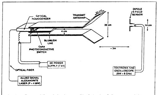
University of Texas at Arlington's impulse transmitter featured an 8-element array of photoconductive switches activated by laser pulses. The resulting electromagnetic pulse propagated down the 4-cm. channel and radiated to free-space. A dipole sensor detected a 400-picosec. wideband field pulse having a peak power of about 800 kw. dah-dah...dah-dah...dah-dah...dah-dah...
