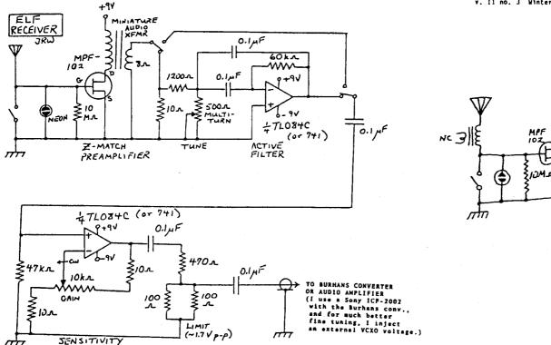
NOTE REGARDING THE FIGURE: The selective element (active filter) shown in this circuit is meant for the 800-1000 Hz frequency range, but its value may be changed to select other audio frequency ranges. See H.M. Berlin, "Design of Active Filters with Experiments," Sams Publications, pl39, 1977.
