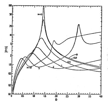
**Figure 2.** The ratio of the horizontal/vertical magnetic fields on the surface over a horizontal buried loop antenna.
