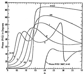
**Figure 3.** The difference in phase between the horizontal and vertical magnetic fields on the surface over a buried loop antenna.
