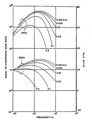
Figure 1. Ratio of magnetic field strength to atmospheric noise on the surface directly over a transmitting loop with magnetic moment of 1000 (amp-turns-sq metres). Receiver bandwidth is 10 Hz. Path lengths of 100 m and 300 m are shown, with ground conductivity of 0.001 - 0.3 mho/m.
