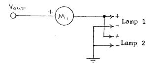
Figure 3. Connecting Multiple Lamps and ammeter
